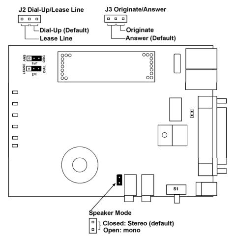
Note: The Speaker Mode Jumper is for the Modem with the Voice Option
